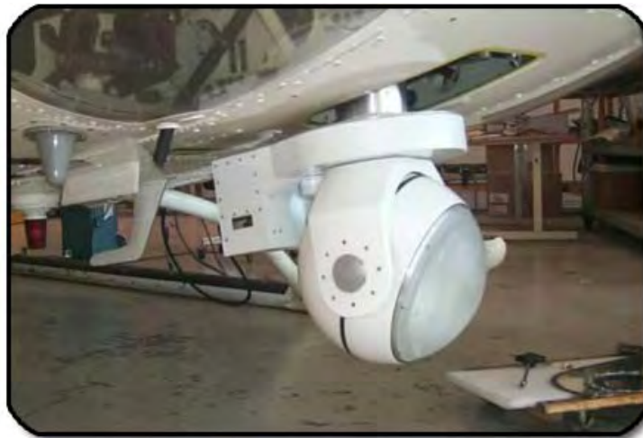
Figure 28. The OASys Scan Head [19]
