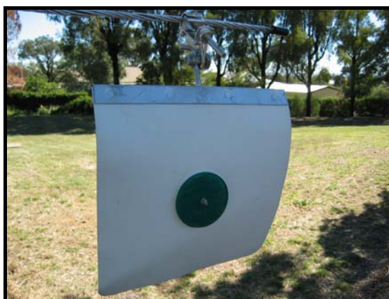
Figure 24. Example of a 'flag marker' used for aerial operations
