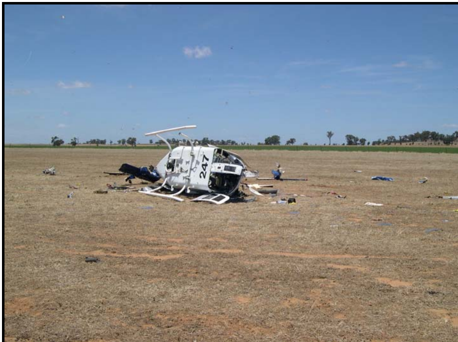
Figure 2. Bell 206B helicopter after striking powerlines during a locust control campaign near Dunedoo on 22 November 2004
