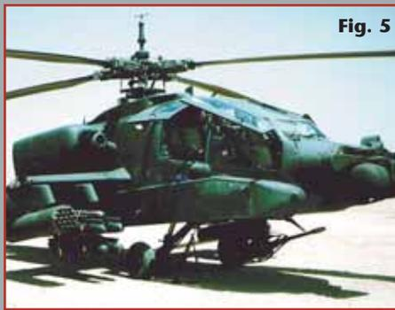
Fig. 5: My Apache in Desert Storm. This picture shows the doors locked in the upright position and the difficulty in someone trying to extract a pilot or quickly egressing the cockpit area.
