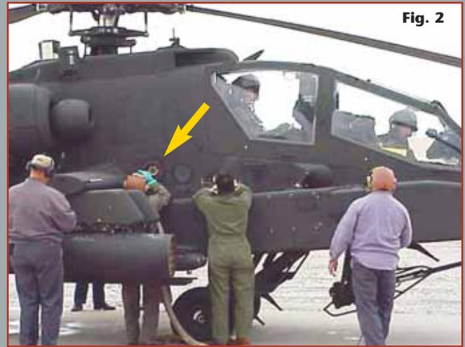
Fig. 2: The pressure refuel point is in the black circle just in front of the wing by the green glove.
