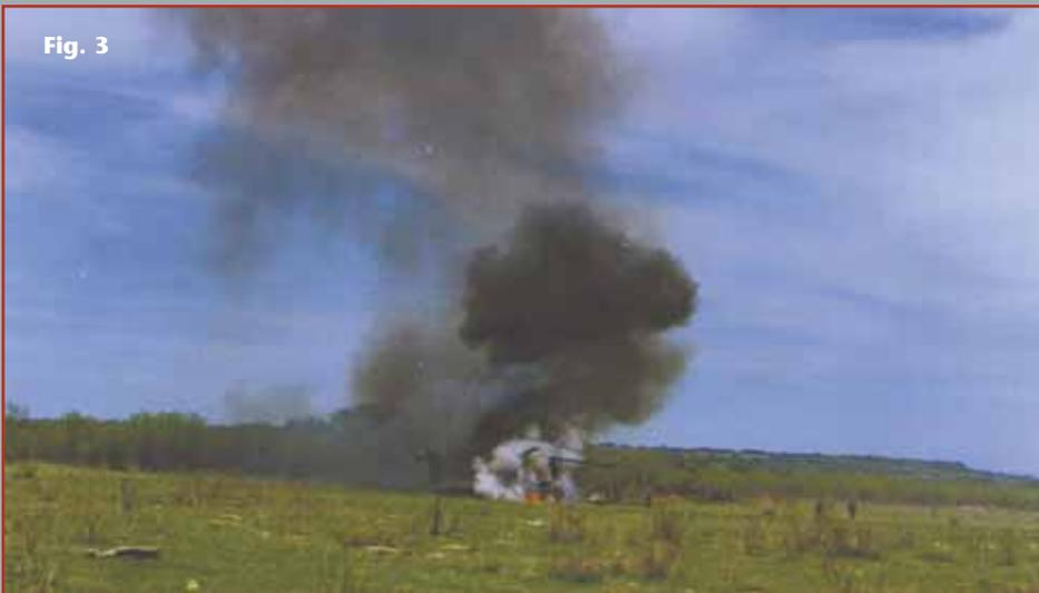
Fig. 3: The vapor cloud has burned off (top smoke) and secondary fires starting from the fuel on the ground and the aircraft.
